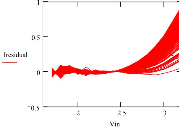
**Figure 5:** Residual current after quadratic fit
