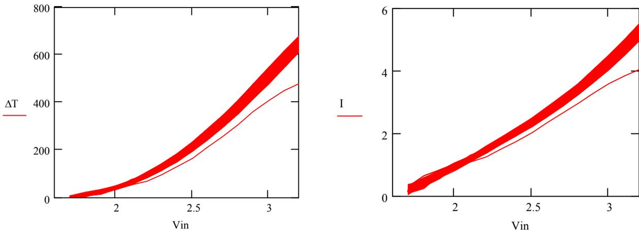
**Figure 4:** Temperature responses and derived current/voltage characteristics (column#2, MSSP array)
