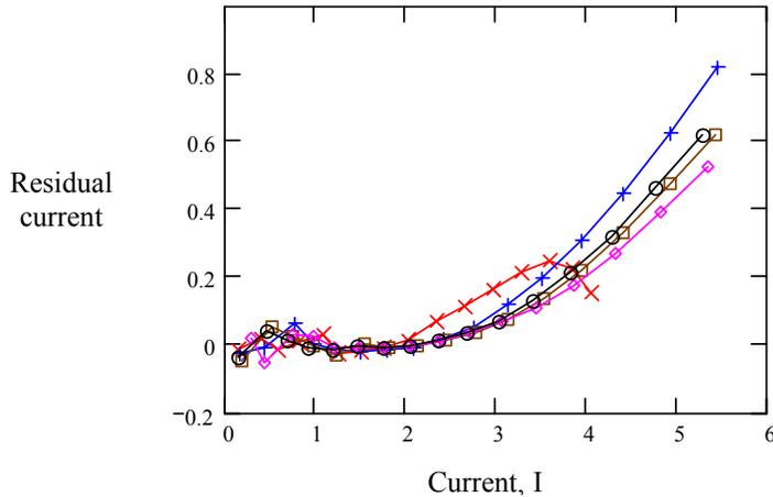
**Figure 6:** Examples of residual current variation with current demand
