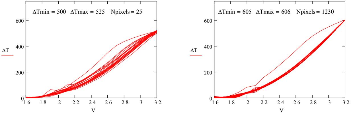
**Figure 3:** Selected temperature responses and 3.2V temperature histogram
