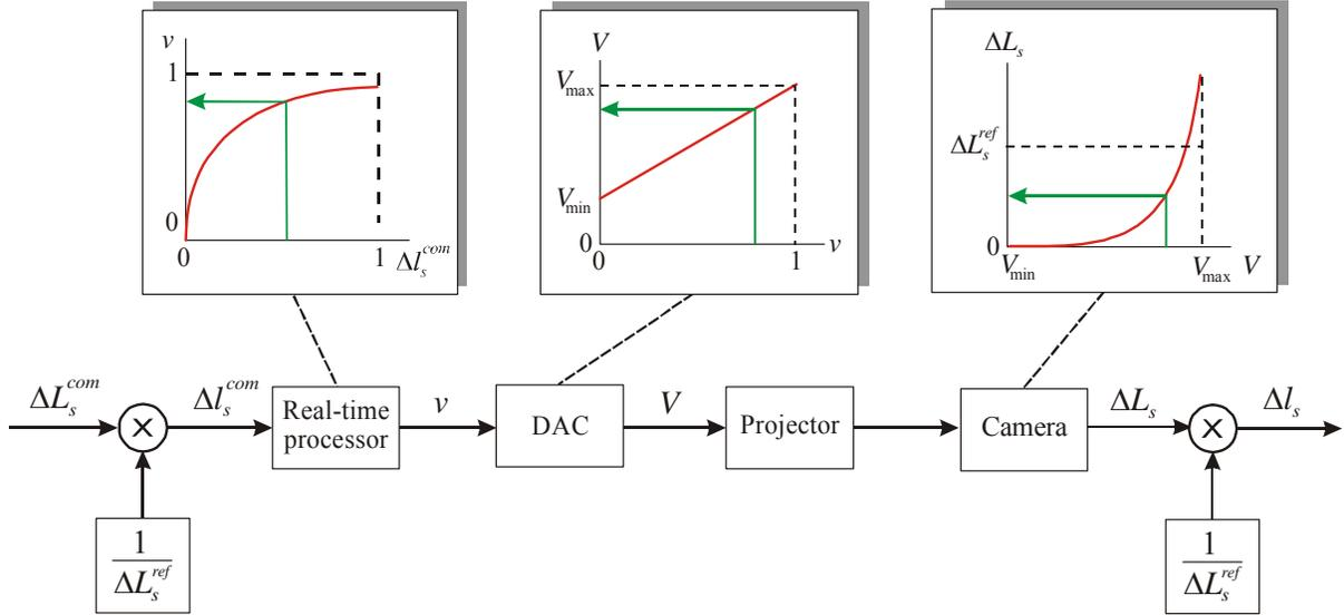
**Figure 1:** Projector scene data transfer (with half maximum radiance command highlighted)
