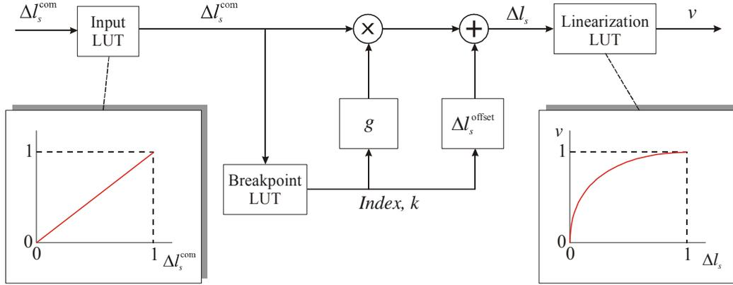
**Figure 2:** Legacy RNUC processor block diagram
