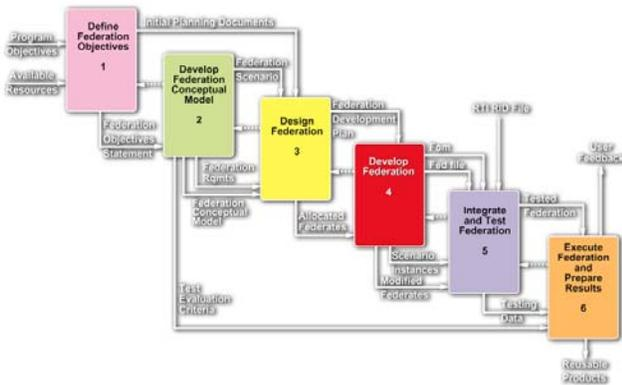
**Figure 2.2.2.1-1 – The Federation Execution Development Process (FEDEP) provides guidance for the composition of simulations into distributed systems**
