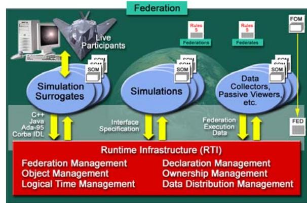
**Figure 2.1.2-1 – The High Level Architecture (HLA) standard provides effective guidance for the interoperation of dissimilar simulations and associated artifacts.**
